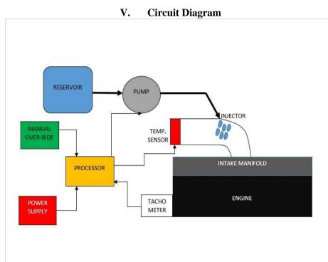
Fig. 4: Circuit Diagram of Water Injection
