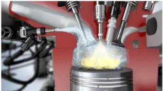
Fig. 2: In-Cylinder Type of Water Injection
